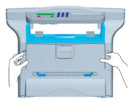
Remove the starter toner cartridge from its bag. Gently roll the cartridge 5 or 6 times to distribute the toner evenly inside the cartridge. Thoroughly rolling the cartridge will assure the maximum copies per cartridge. Hold it by its handle.
